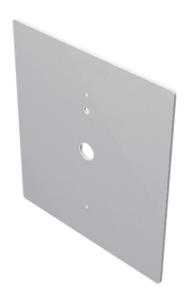
Plate for the installation of the Visto smart doorbell on existing recessed boxes type 503 (horizontal and vertical) with interaxis of 83.5mm, square boxes with interaxis of 62mm, box type 502/German/round with interaxis of 60mm. Made of PMMA, white color.
