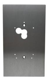
Plate allowing installation of the Extra, Ciao and Quadra external units in 1- and 2-module flush-mounted boxes by Comelit, Bticino and Urmet. Dimensions (LxHxP): 137x236x2.5 mm.
