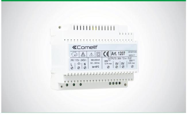
Power supply unit with overload and short circuit protection devices. It has two separate continuous outputs: one to power the external unit and electric lock, and the other to power the monitor. Input voltage 120-230 VAC. Dimensions: 105x85x85 mm (6 DIN modules).
