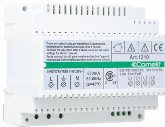
2-wire power supply unit required to power the external unit (terminals L1 - L1) and the support column (terminals L2 - L2). Equipped with 1 terminal for line termination art 1216. Input voltage 110-240Vac. Compatible with audio/video unit art. 4681 and 1621VC and audio unit art. 1621. Dimensions: 106x89x62mm (6 DIN modules).
