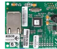
**Plug-in GSM/GPRS Module**
